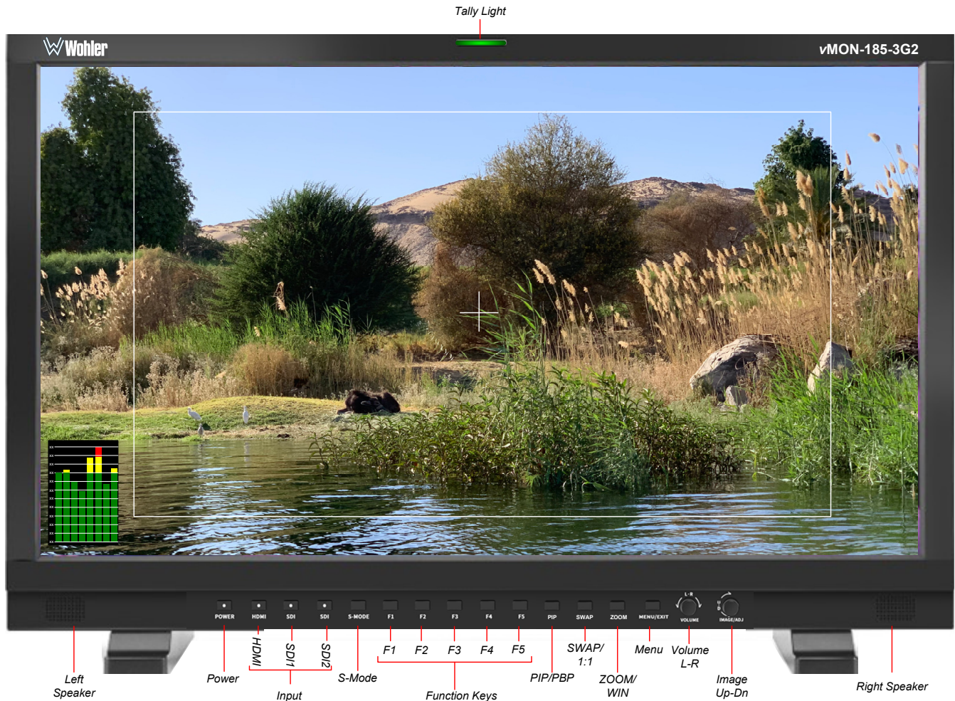
Figure 2-2: vMON-185-3G2 Front Panel
